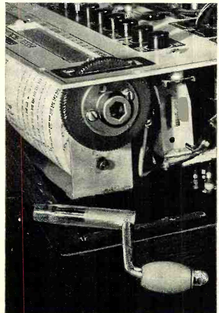
Fig. 3. Roll chart assembly lifted out of case to show how crank mount is added.
